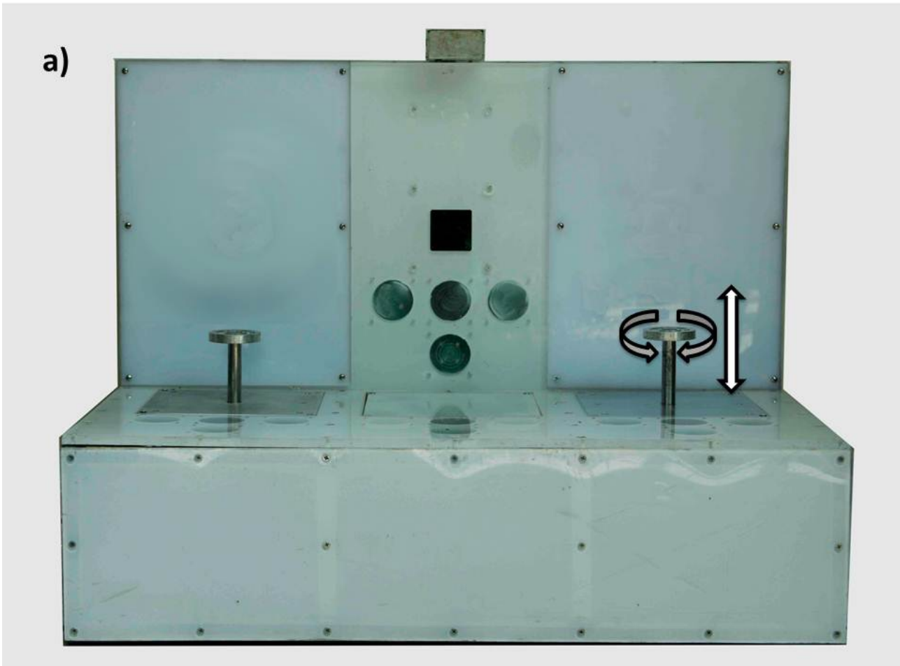
Fig 1 The mechatronic board. The modules are on the right and left sides of the platform, whereas the black square in the vertical central panel is the opaque rewarding box. The circles below the box could light while the ones close to the modules could produce sounds. The grey arrow shows the rotation of the tap and the white arrow the lifting of the bar.
